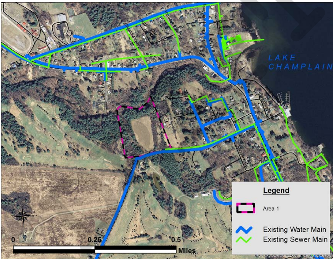
Figure 5. Existing sewer and water infrastructure near Area 1 shown on an aerial image.
