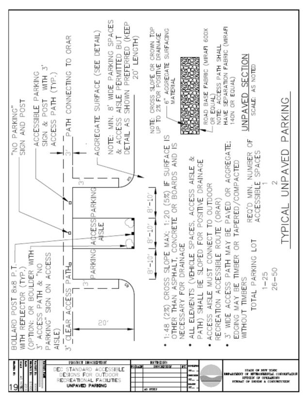
Figure 10. Typical unpaved accessible parking details.
