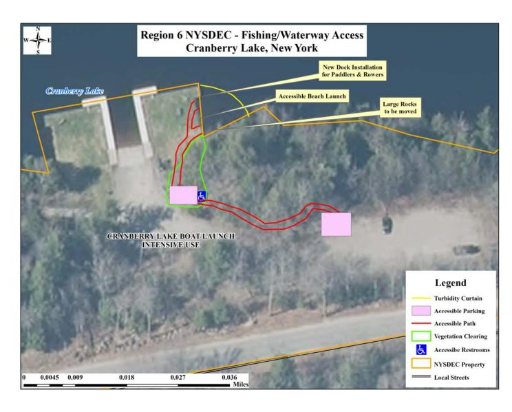
Figure 3. Orthoimagery map of the existing Cranberry Lake BLS with site plan details.
