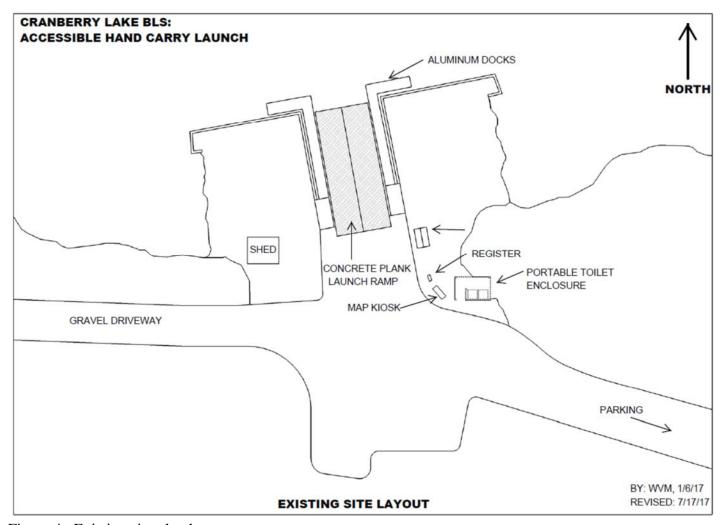
Figure 4. Existing site plan layout.
