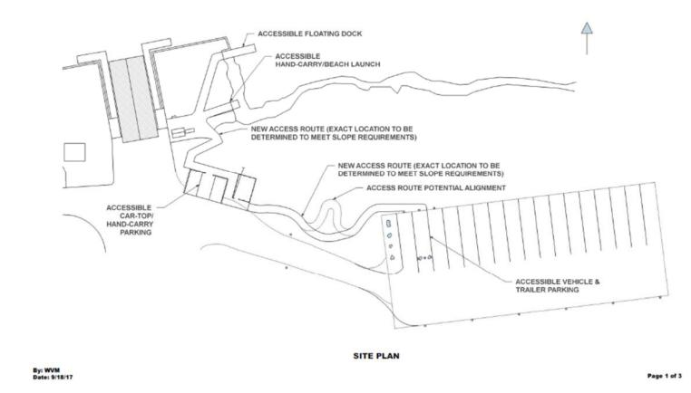
Figure 5. Site plan details for the construction of the accessible beach launch and accessible parking at the Cranberry Lake BLS.
