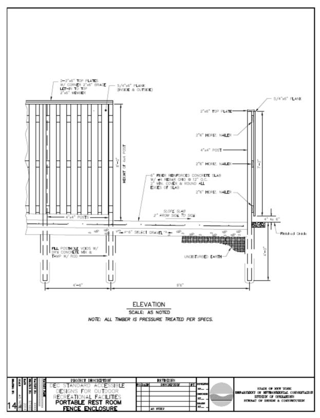
Figure 9. Portable restroom fence enclosure details (continued).
