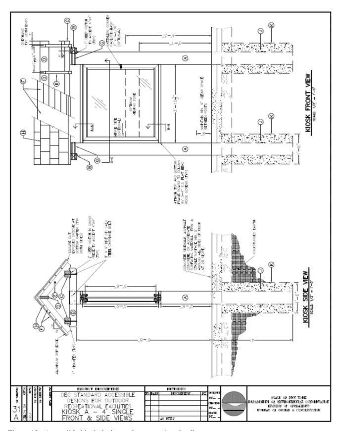
Figure 12. Accessible kiosk design and construction details.
