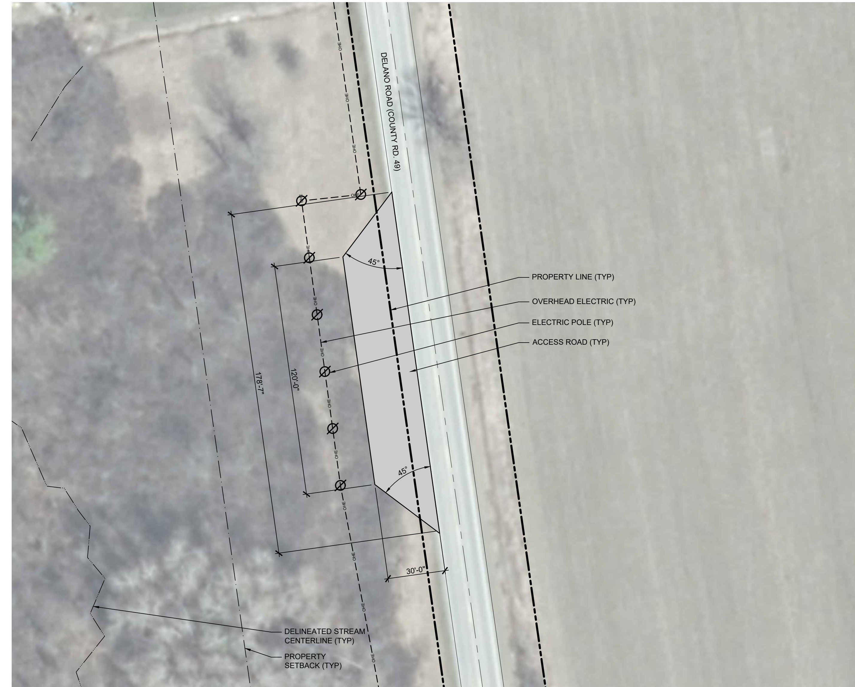
2 ELECTRIC POLE PULL OFF AREA ENLARGEMENT Scale: 1" = 30'
