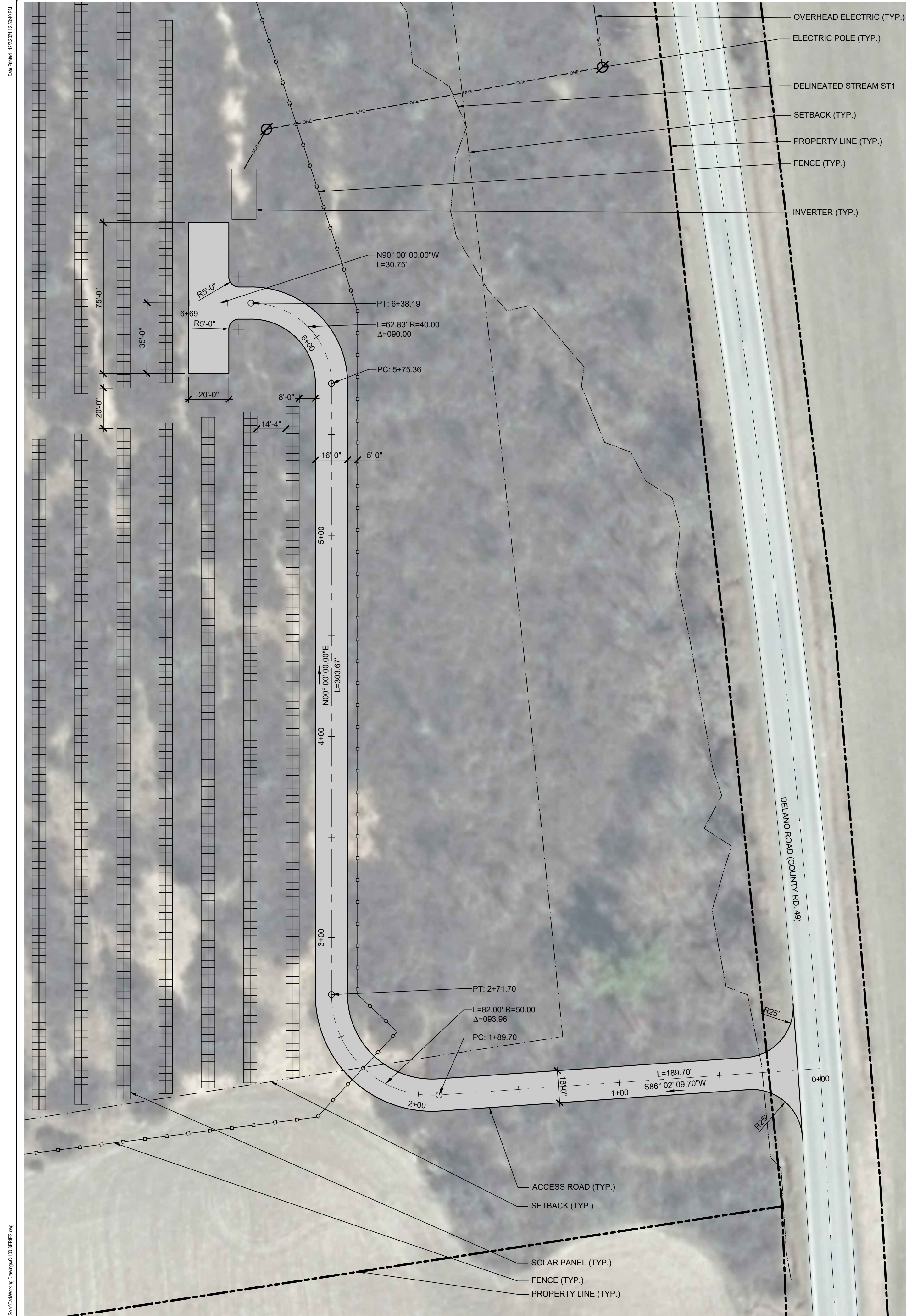
1 ACCESS ROAD ENLARGEMENT PLAN Scale: 1" = 30'
