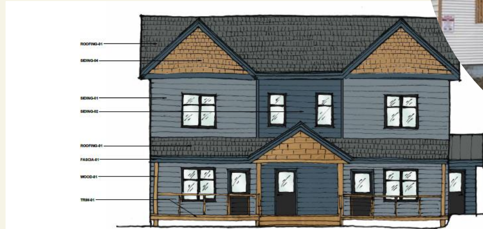
2 NORTH ELEVATION A202 1/4" = 1'-0" ON 22'x34"
