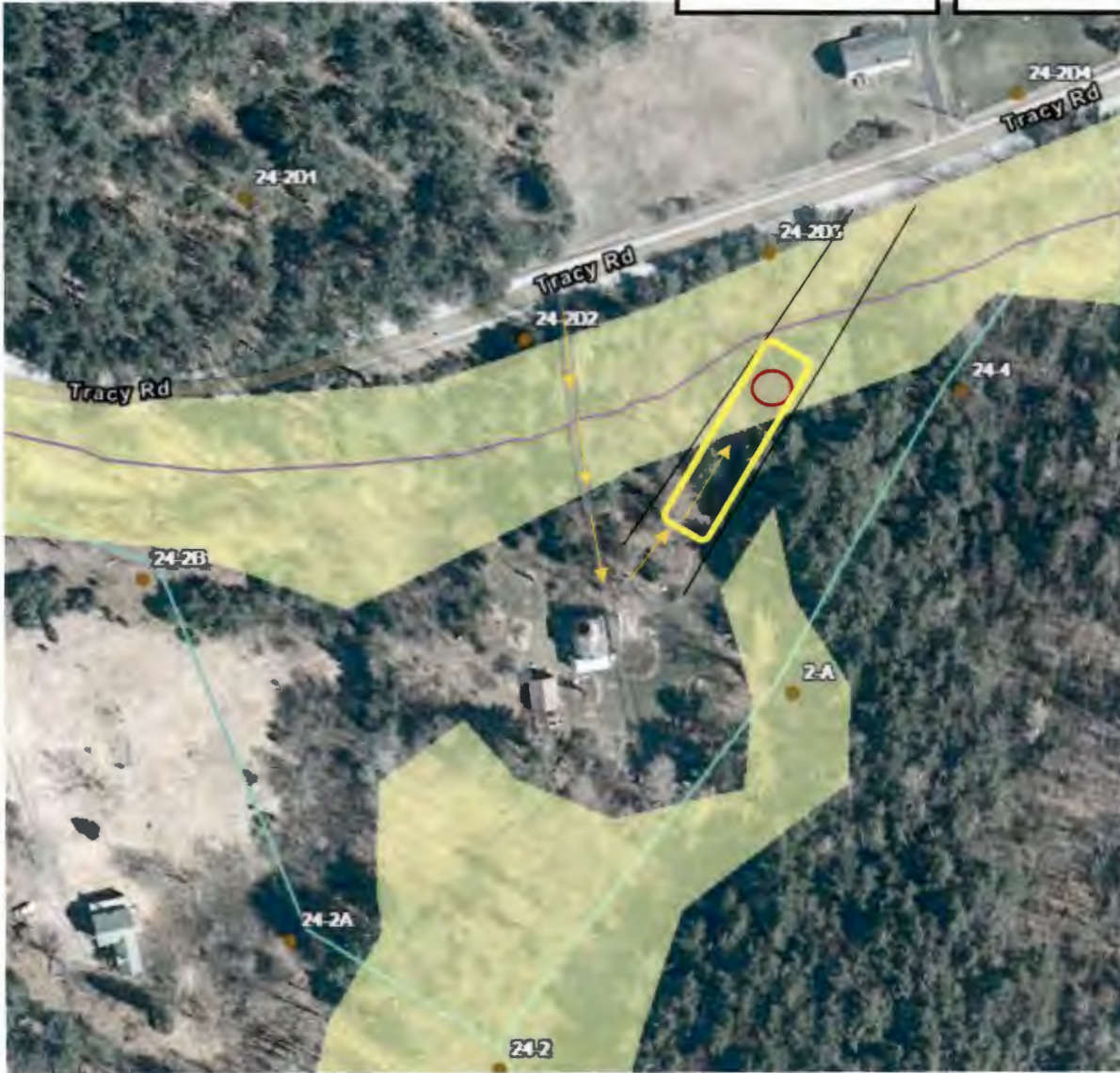
Structure 24-4 (depicted by the red circle) will be accessed via the driveway at 1554 Tracy Road and on the utility right of way (black line), as indicated by the orange arrows. The area highlighted by the yellow rectangle indicates potential area for timber mat placement and/or minor low grow brush trimming.
