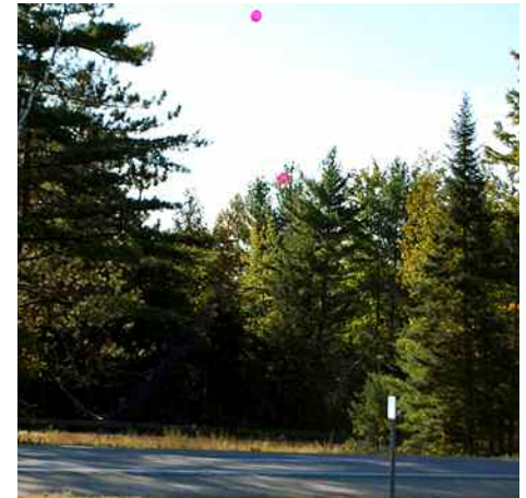
As part of visual analysis, balloons are floated above a proposed project site to help determine substantial invisibility.
