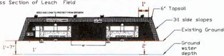
Cross Section of Leach Field
