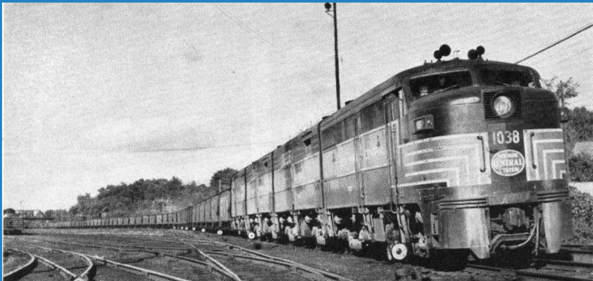
FOUR MIGHTY UNITS of diesel power pull the ore train. Usual consist on this run is 65 to 70 cars, each loaded with about 55 tons of ore. Picking its way out of Benson Mines yard, train is seen here at start of its daily run to Watertown, then on to the Central's Belle Isle yard.
